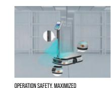
360° obstacle avoidance, anti-collision strip, and 3 emergency
