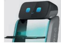
SAFETY, ELEVATED DINERBOT T9 Pro uses stereo vision sensors for precise, safe service in any environment. Made possible by tray sensors, and voice and visual guidance.
